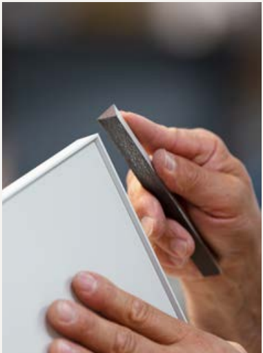
Meticulous work right to the finish. The corners are deburred by hand using a grindstone for a perfect result, both visually and tactilely.
